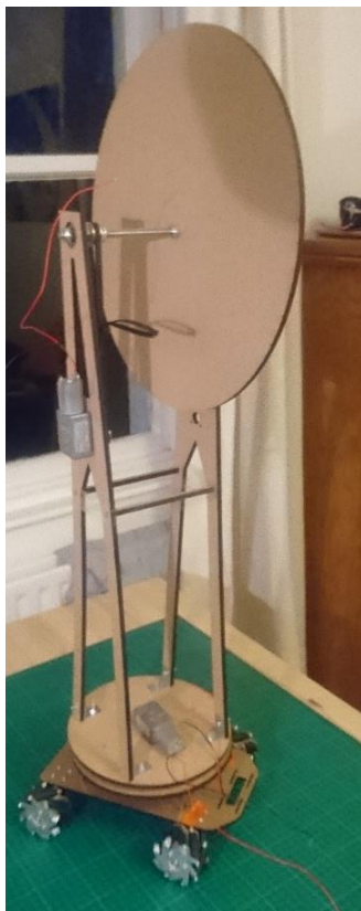
Figure 32: The new DC motors attached to the axle mount and the base plate.
