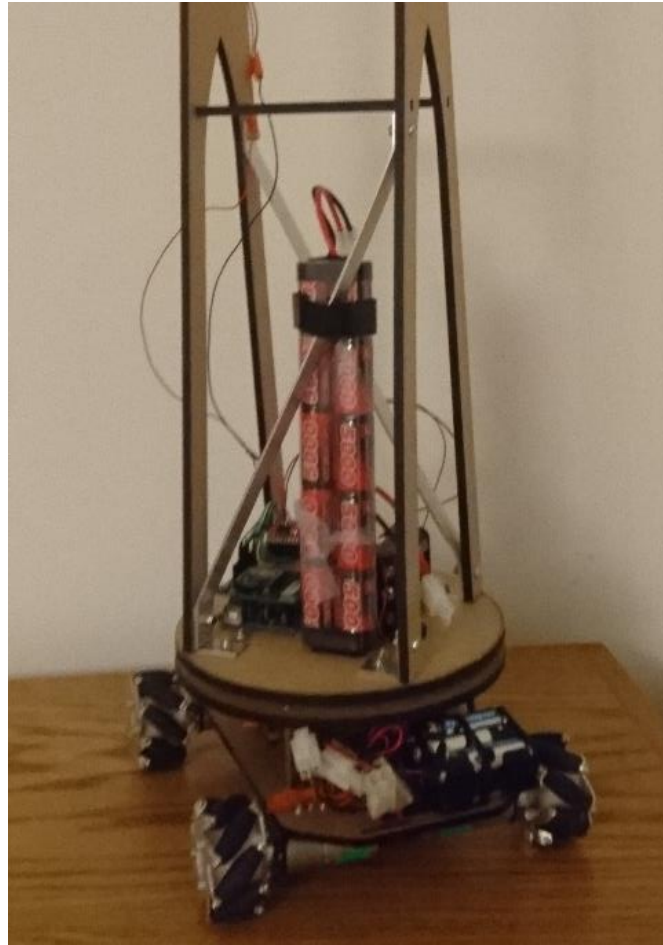
Figure 33: Assembly with angled struts
